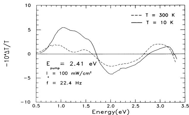
FIG. 2. Near-steady-state photoinduced absorption spectra of PNB cast on quartz substrate.
