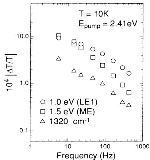
FIG. 4. Chopper-frequency dependence of the 1.0 eV, 1.5 eV, and  $1320\text{ cm}^{-1}$  transitions of PNB. The data of the 1.0- and 1.5-eV peaks were taken on thin-film samples with  $I_0=100$   $\text{mW}/\text{cm}^2$ ; those of the  $1320\text{ cm}^{-1}$  transition were taken on a pressed pellet of PNB mixed with KBr and  $I_0=250\text{ mW}/\text{cm}^2$ .
