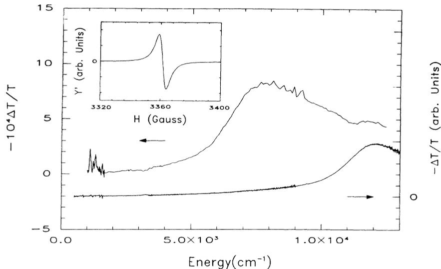
FIG. 3. Photoinduced absorption spectra of PNB as powder mixed with KBr, obtained with pump laser intensity  $I_0=250$   $\text{mW}/\text{cm}^2$ . Left scale: Near-steady-state (22.4-Hz light modulation) at 10 K. Right scale: Long-lived (reduced by a factor of  $\sim 400$ ) at 80 K. Inset: LESR derivative signal after the sample was exposed to a laser beam ( $E_{\text{pump}}=2.54$  eV,  $I_0=100$   $\text{mW}/\text{cm}^2$ ) for 1 h and at 60 K.
